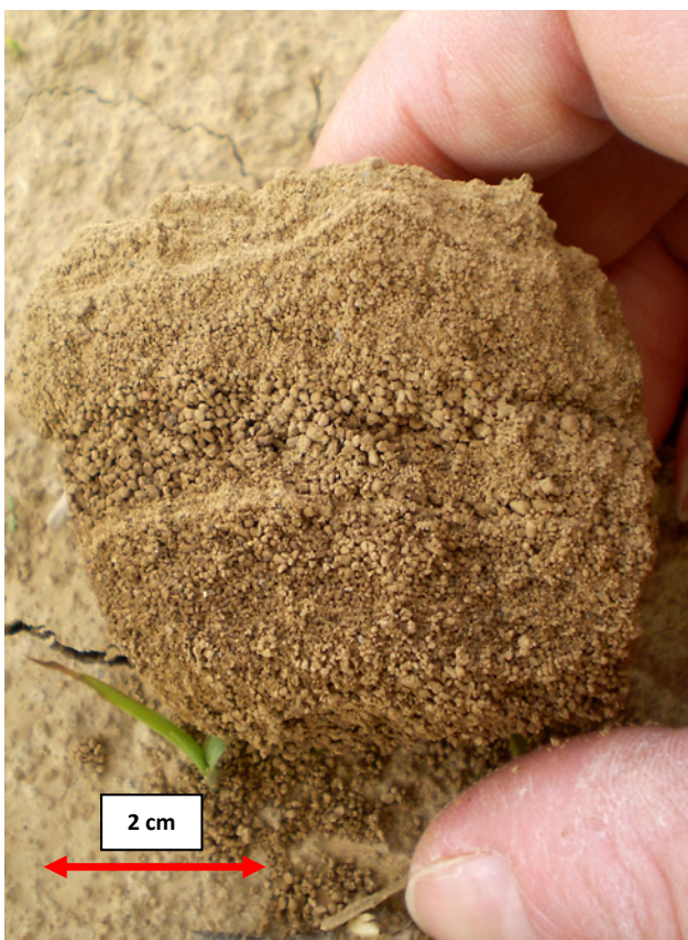
Figure 3 Layers of grain size in soil crust
