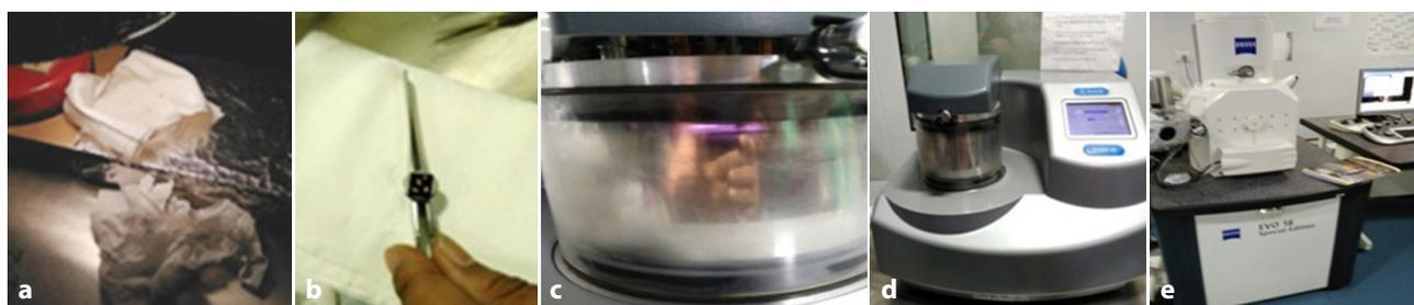
**Figure 1** Specimen coating and imaging in scanning electron microscope (Carl Zeiss EVO 18)
