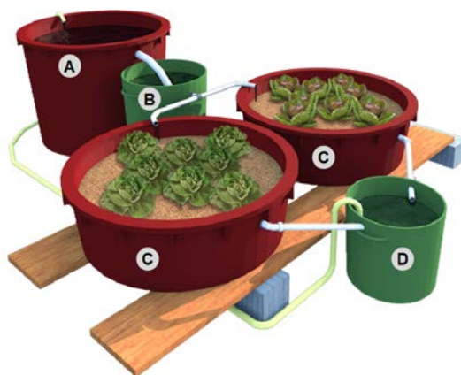
Figure 1 Rendering of the aquaponic unit. A, main tank for fish (500 L); B, settling vessel (100 L); C, tanks for vegetables/biofilters (275 L); D, storage tank for water collection (50 L) and pumping to A tank
